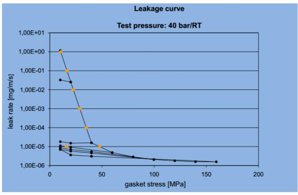
Diagram of a tightness test of a gasket 92 x 49mm cut out of 3mm ePTFE sheet, test gas pressure 40 bar. X axis - stress applied on the gasket in MPa Y axis - specific leak rate, where 1 мg/m/s corresponds to tightness level L1 Example: tightness level is L0,01 is achieved when gasket stress 22 MPA is applied.
